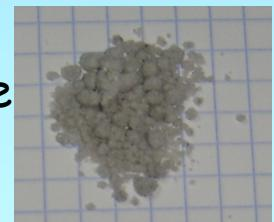
Continuous deposition on particles of bed material, and depending on the melting behavior of these deposits, it can occur partial melting and agglomeration.
