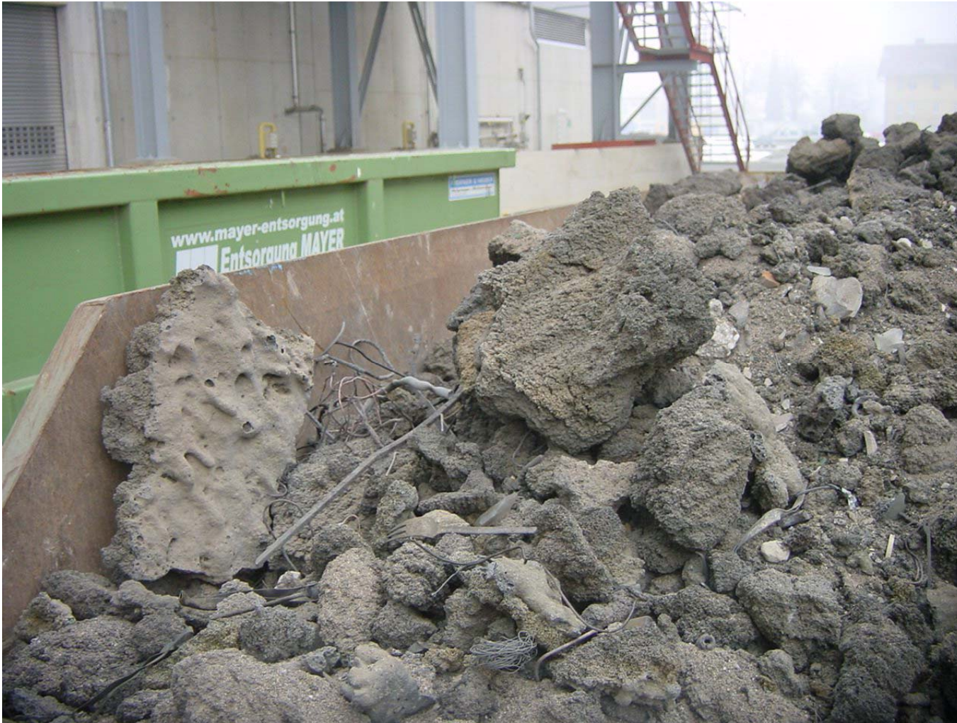
Slag Removed from Furnace
