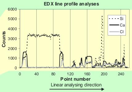
EDX line profile analyses of Si, Ca and Cl for a sample of SiO $_2$  and CaO reacted with HCl, O $_2$  and N $_2$  at 850°C. Reaction time: 90 min.
