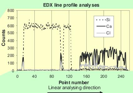
EDX line profile analyses of Si, Ca and Cl for a sample of SiO $_2$  and CaO reacted with HCl, O $_2$  and N $_2$  at 850°C. Reaction time: 10 min.
