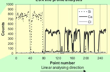
EDX line profile analyses of Si, Ca and Cl for a sample of  $SiO_2$  and CaO treated in  $O_2$  and  $N_2$  at  $850^{\circ}C$ . Reaction time: 90 min.
