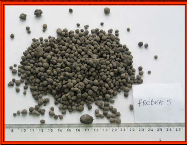
Fuel 5: granulated coal with addition of sewage sludge (H-34)
