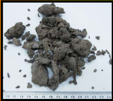
Waste from paper mill facility (dried sludge from waste-paper discolourization)
