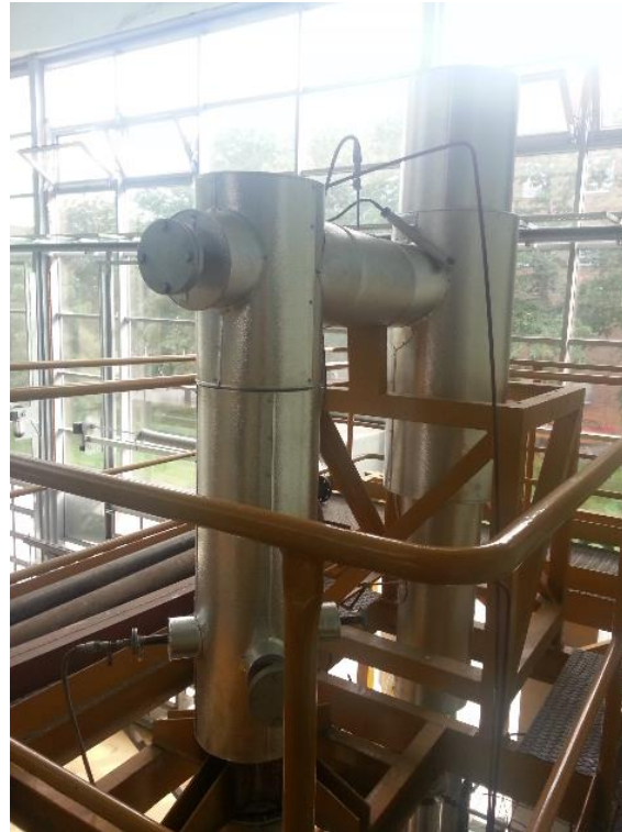
Riser, Cyclone int. \varnothing 219 mm
