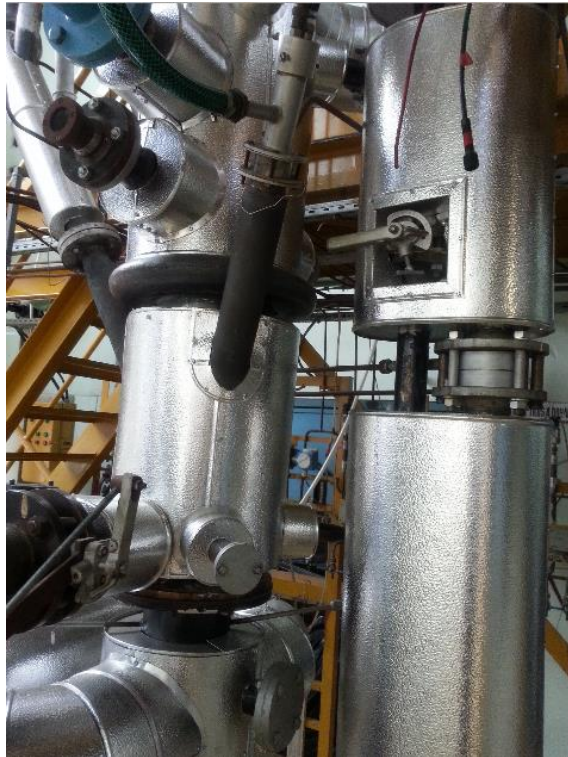
Riser height: 5 m int. \varnothing 158 mm
