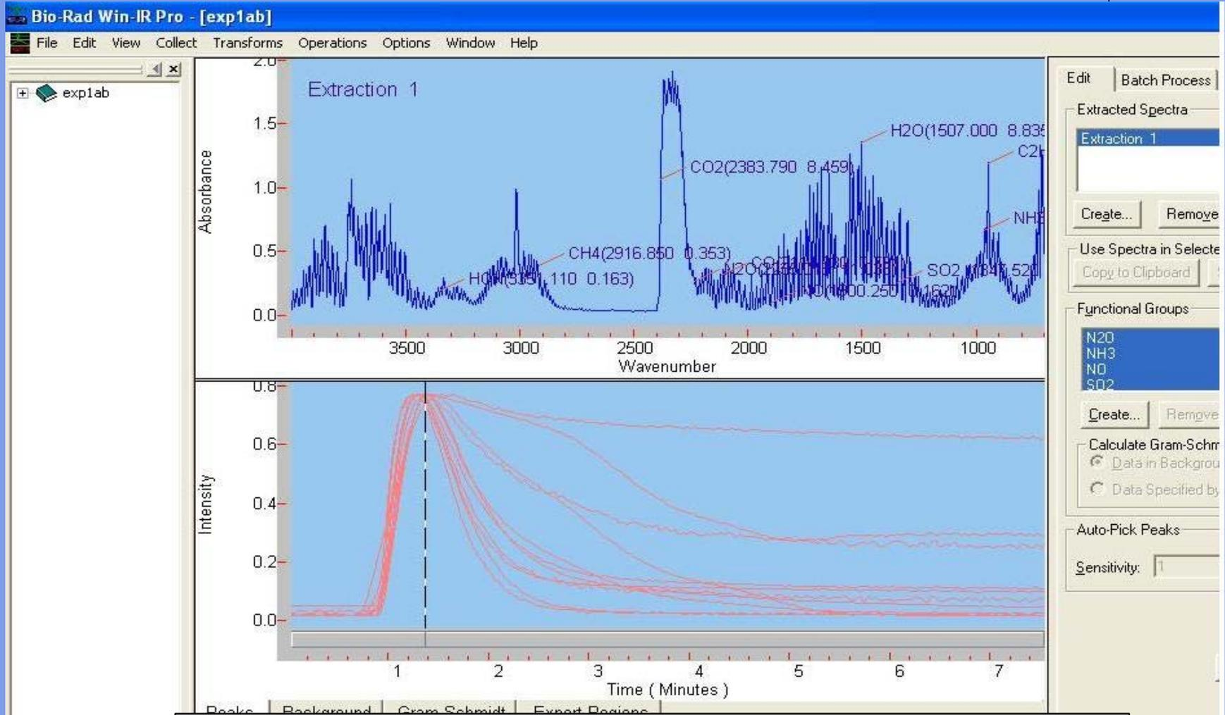
*Spectrum obtained from leather combustion at 800°C and 6 % O<sub>2</sub>*
