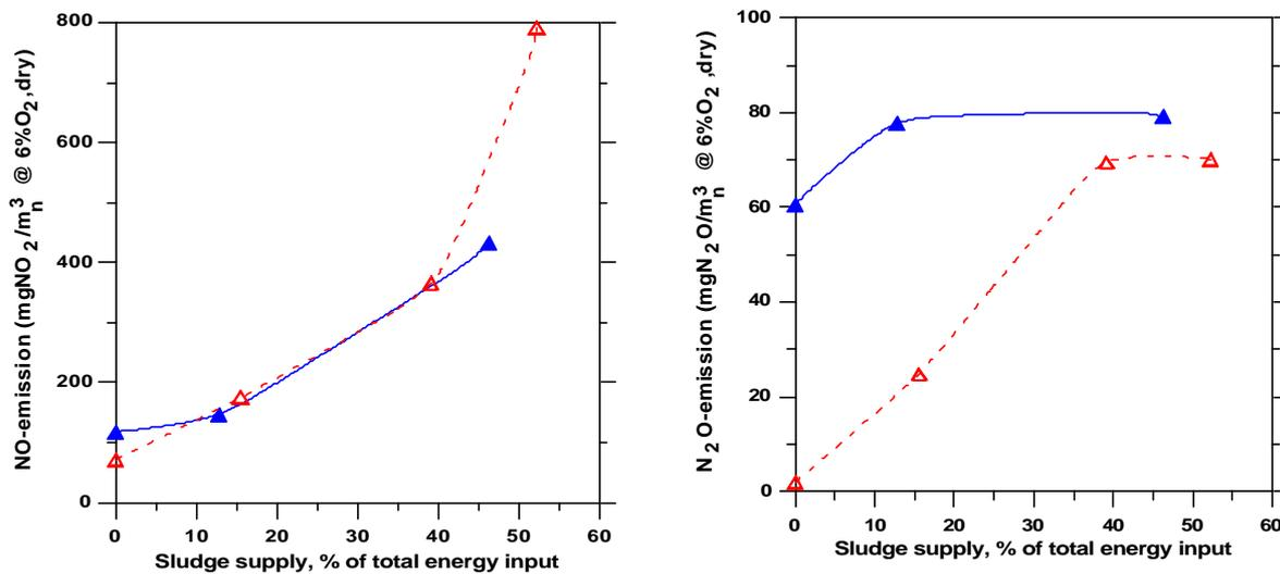
**Fig. 2** Emissions of NO and N<sub>2</sub>O during advanced air staging
