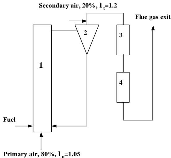
**Fig. 1.** CFB combustor showing “advanced” air staging. 1 Combustion chamber, 2 Particle separator, cyclone, 3 Afterburner, 4 Convection path.
