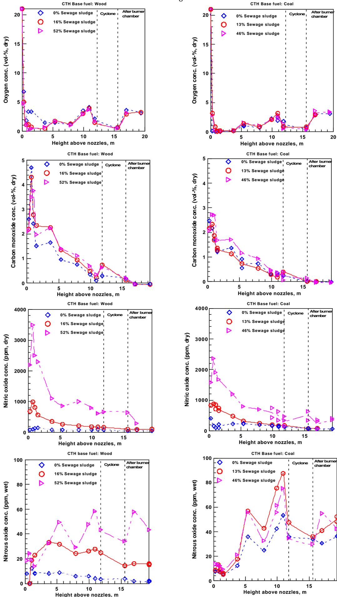
**Fig. 4.** Concentrations of O<sub>2</sub>, CO, NO, and N<sub>2</sub>O on the centre-line of the CTH boiler during co-combustion of coal or wood with dried sewage sludge. Advanced staging.
