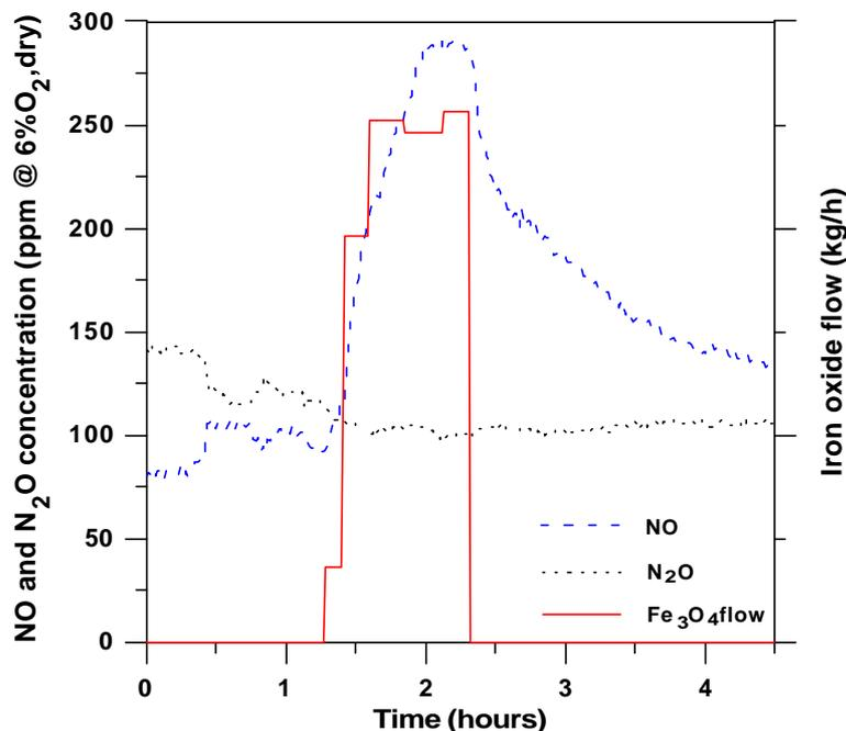
**Fig. 5** Addition of iron oxide (Fe<sub>3</sub>O<sub>4</sub>) to the CTH combustion chamber during combustion of coal under normal operating conditions. Between t=1.42 and t=2.30 the average iron oxide addition is 485 kg/h which is equal to 2.8 kmol/h.
