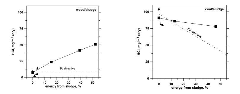
Wet  $\blacktriangle$  and dry  $\blacksquare$  sludge with wood and coal as base fuels compared with the EU directive completed with local regulations. Advanced staging.
